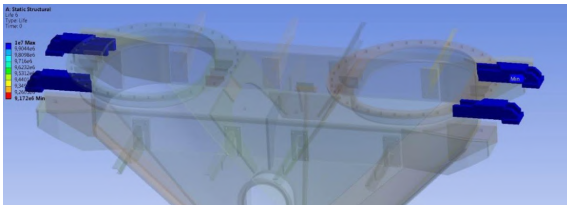
Fig. 2.16 Distribution of lifespan of centering unit's supports by Wehler SN curve
