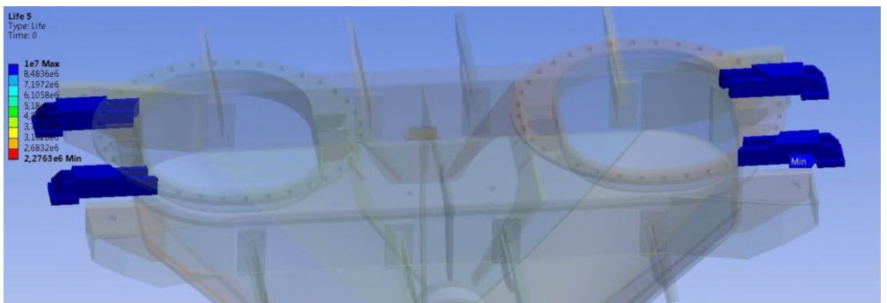
Fig. 2.56 Distribution of lifespan of centering unit's supports by Wehler SN curve.
