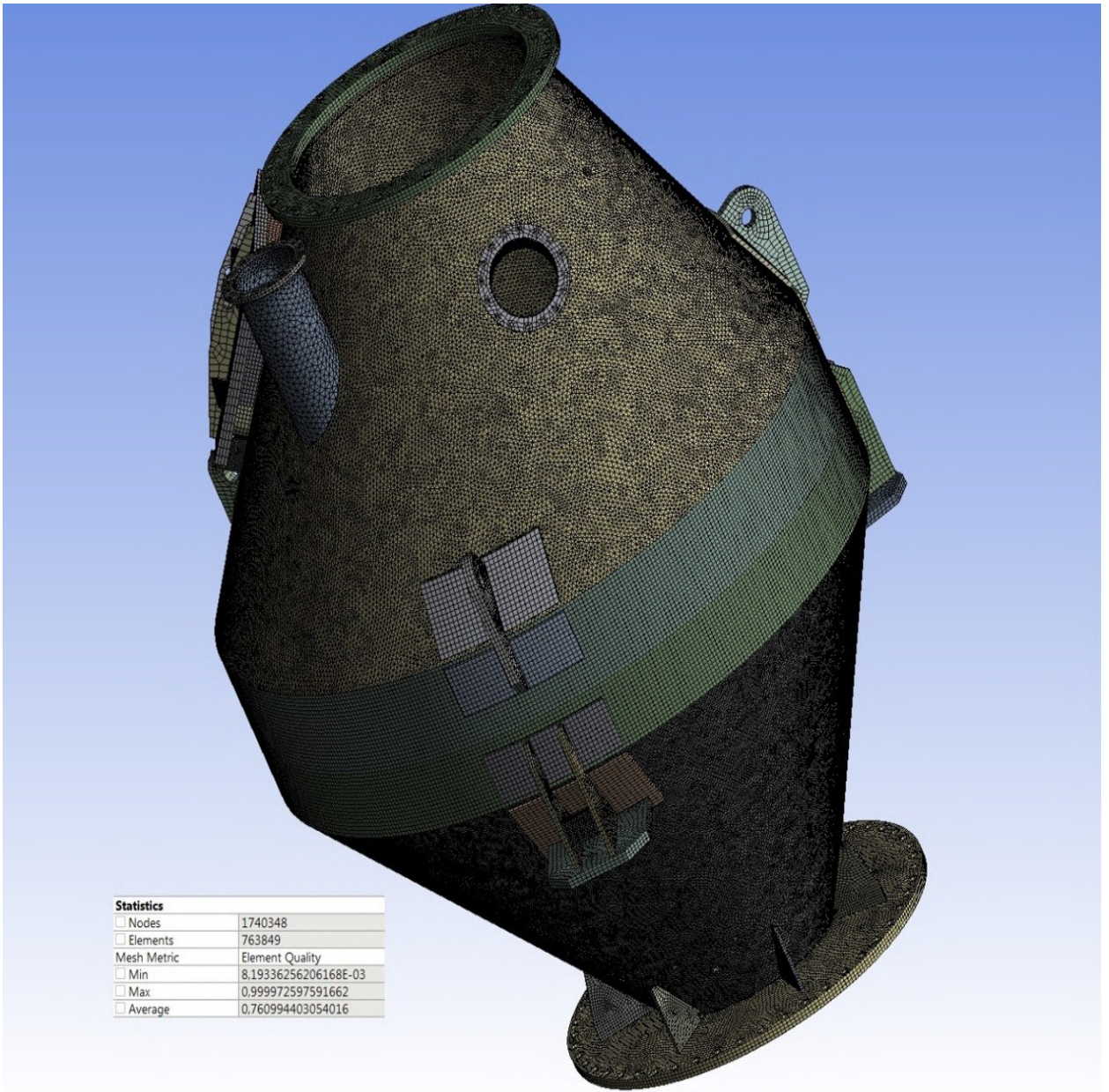
Fig. 1.5 Finite-element model for material bin designing
